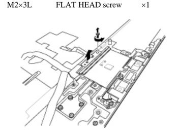
Figure 4-24 Removing screw securing touchpad on-off board
